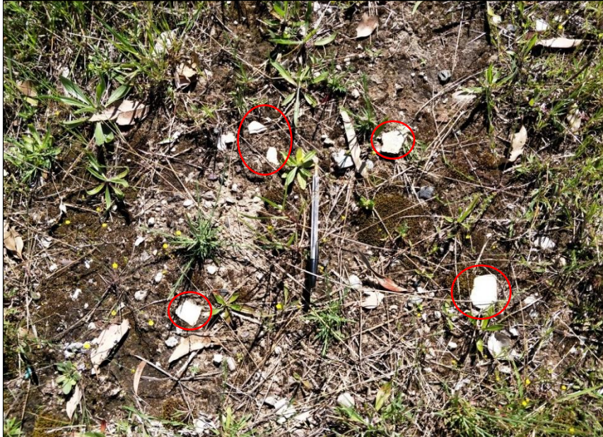
16: POTENTIAL ACM FRAGMENTS ON GROUND SURFACE OF HISTORICAL COTTAGE AREA. POTENTIAL ACM FRAGMENT IS CIRCLED
